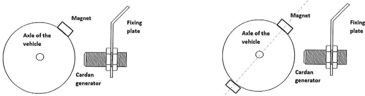
The maximum distance between the magnets on the drive shaft and the sensor is 10 mm.
